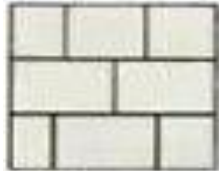
Ashlar stone masonry
