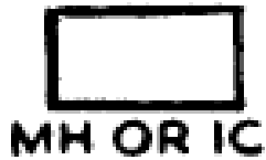
Both Man hole and Inspection chamber
