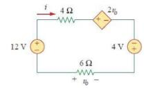
8. Use mesh analysis to find the current in the given circuit
