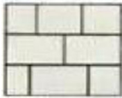
Ashlar stone masonry
